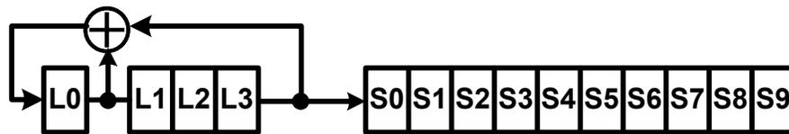
Figure 3.1 An LFSR connected to a scan chain of 10 flip-flops.
