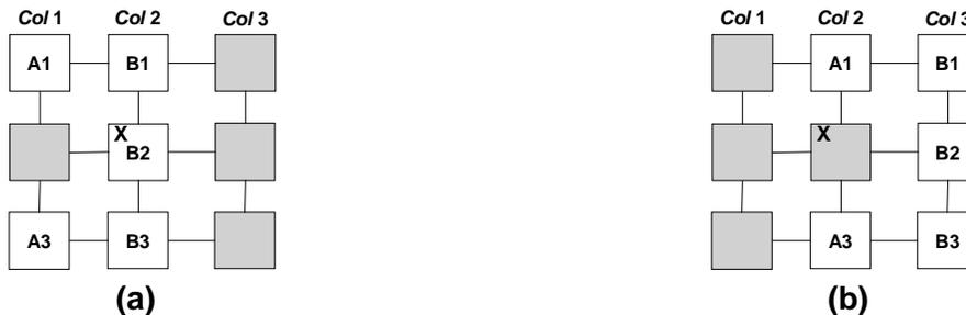
**Figure 6-2: Unidentified fault location. (a) Original. (b) Alternative configuration. (Shaded area represents unused elements.)**
