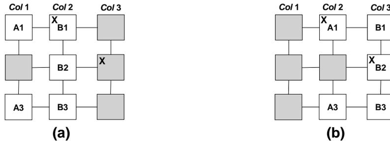
**Figure 6-1: Effect of dormant faults. (a) Original. (b) Alternative configuration. (Shaded area represents unused elements.)**
