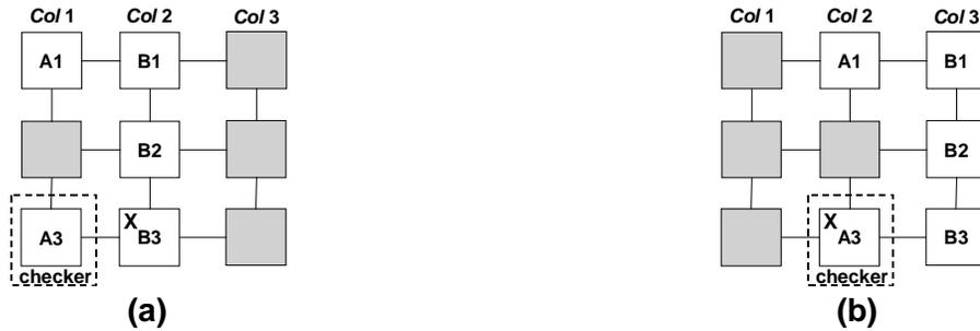
**Figure 6-3: Effect of reconfiguration order. (a) Original. (b) Alternative configuration.**
