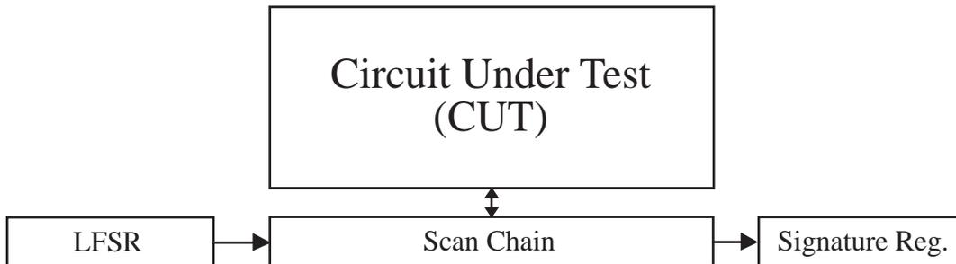
Figure 3.1. Block Diagram for Serial BIST Scheme ("Test-Per-Scan")
