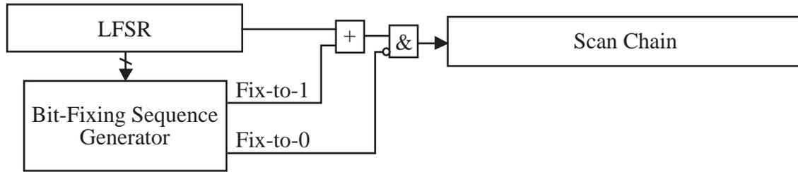
Figure 3.5. Logic for Altering the Pseudo-Random Bit Sequence
