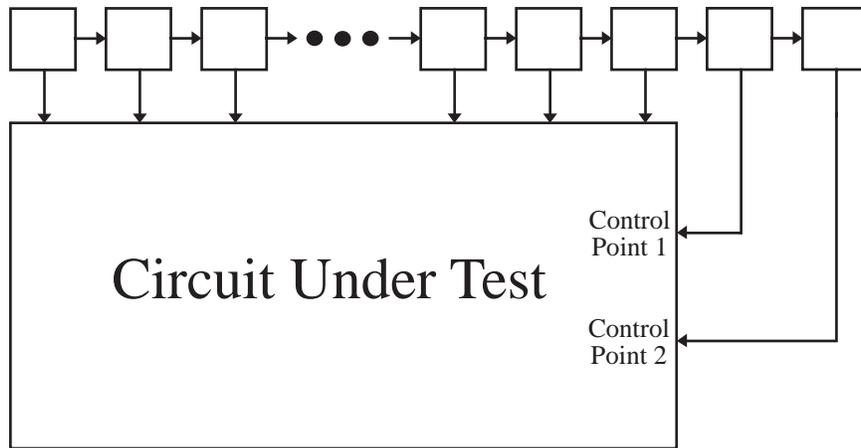
Figure 2.4. Control Points Driven by Extra Scan Elements
