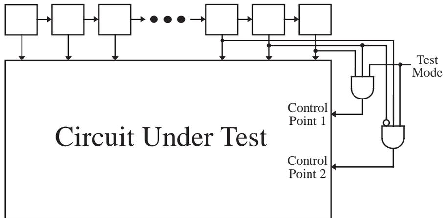
Figure 2.5. Control Points Driven by Pattern Decoding Logic
