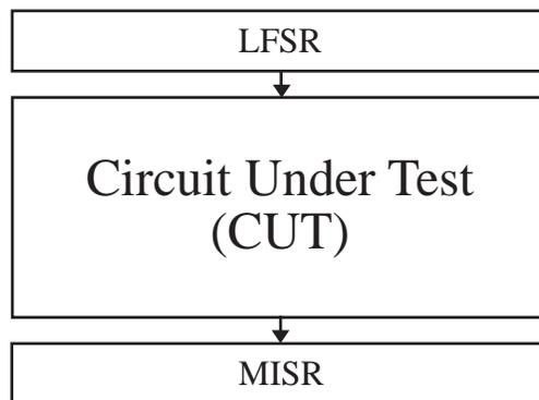
Figure 3.2. Block Diagram for Parallel BIST Scheme ("Test-Per-Clock")
