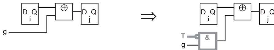
**Figure 7. Case X flip-flop before and after test logic is inserted**
