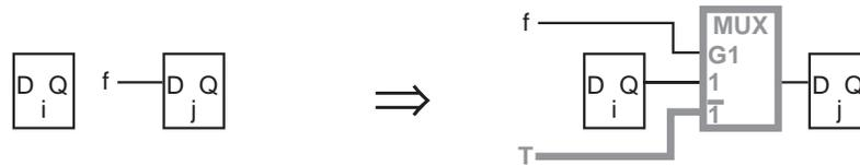
**Figure 10. Case N or case O flip-flop before and after test logic is inserted**
