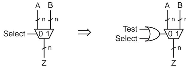
Figure 3-7. Multiplier with modified select signal
