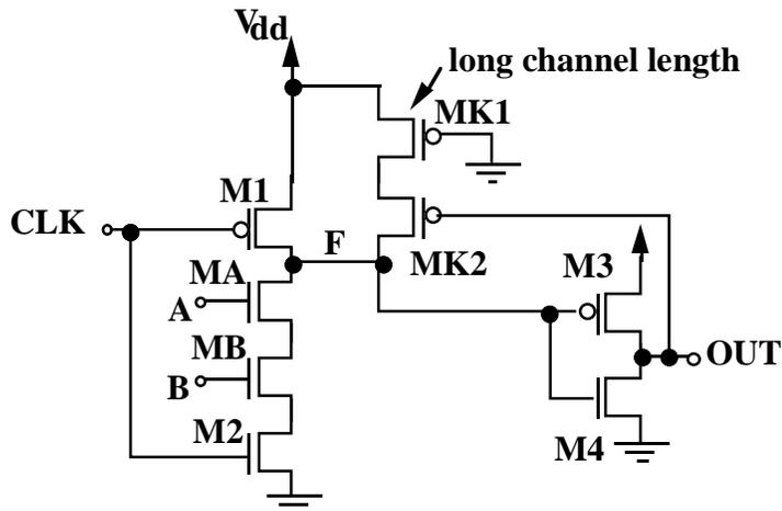
**Figure 4-9 Keeper Design C in a Tiny CMOS Domino Circuit**
