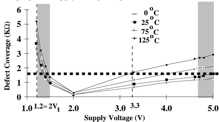
**Figure C-10 Desired Supply Voltage Range (in the Gray Region) When G2 and G3 in Fig. C-6 are 4-Input AND Gates**
