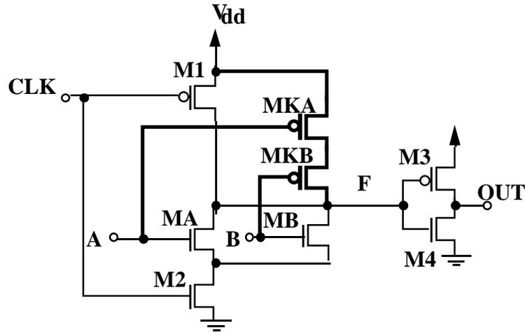
**Figure 4-8 2-input CMOS Domino OR Gate with Keeper Design A**
