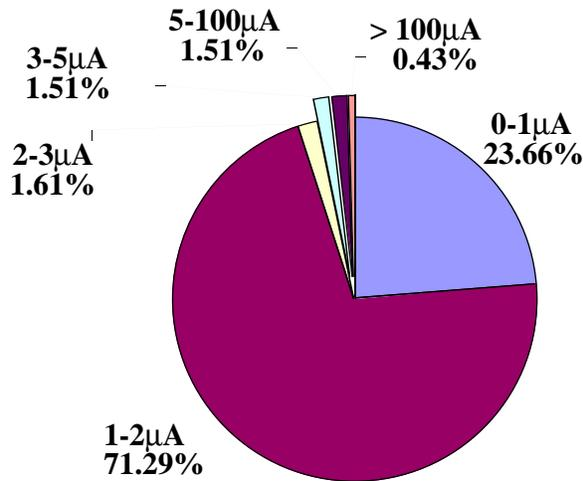
**Figure 6-4 Maximum  $I_{DDQ}$  Distribution of the 930 CUTs that Passed All the Boolean Tests at Nominal Voltage for IDDQ1 Test Set**
