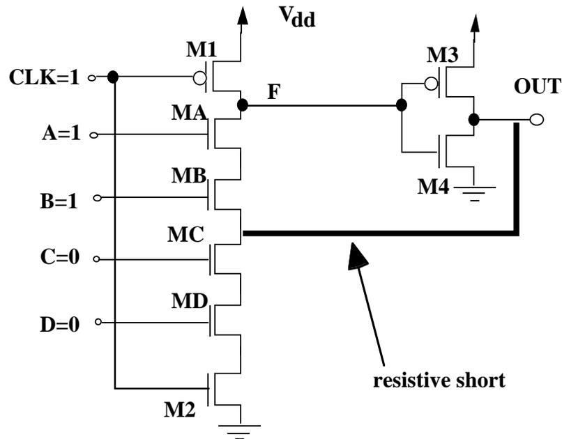
**Figure C-5 An SHI between the Output Node and the Source Node of an NMOS Transistor in the Evaluation Network**
