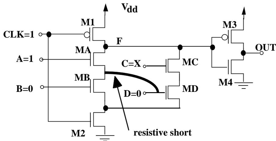
**Figure C-4 An SHI between an Input Node and the Source Node of an NMOS Transistor in the Evaluation Network**
