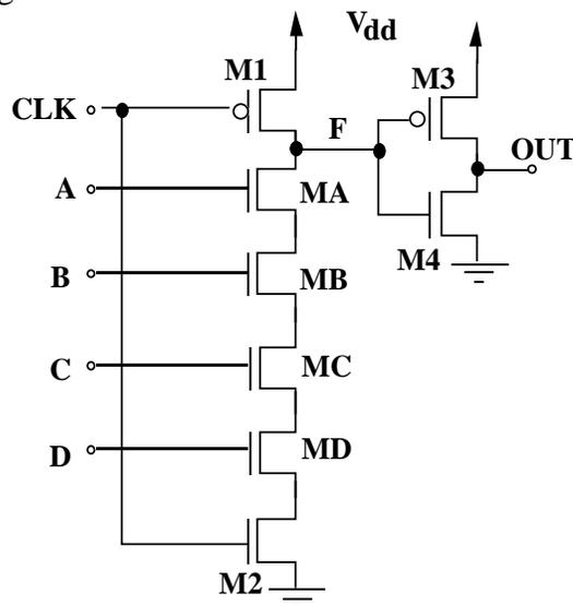
Figure C-1 4-Input AND Gate
