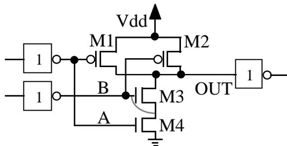
**Figure 2-1 NMOS Gate Oxide Short**
