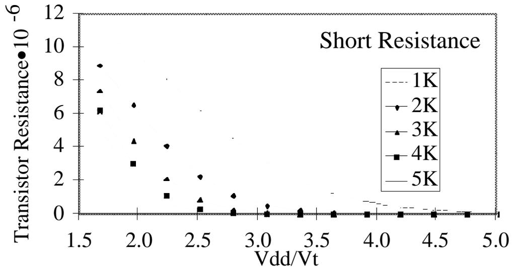
**Figure 2-2 The Equivalent Resistance of a Defective NMOS Transistor for a 0.8  $\mu\text{m}$  Technology**
