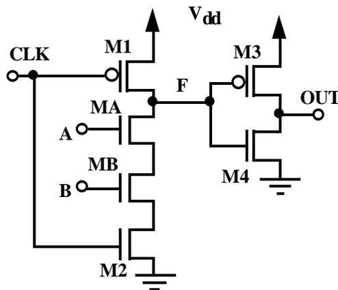
Figure 4-1 CMOS Domino Circuit
