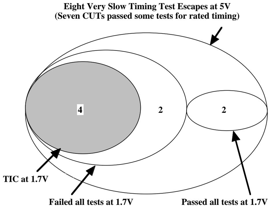
**Figure 6-5 VLV Test Results for CUTs with Very-Slow Timing Test Escapes**
