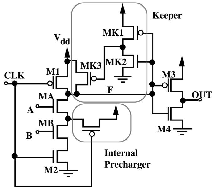
Figure 4-2 CMOS Domino Circuit with a Keeper
