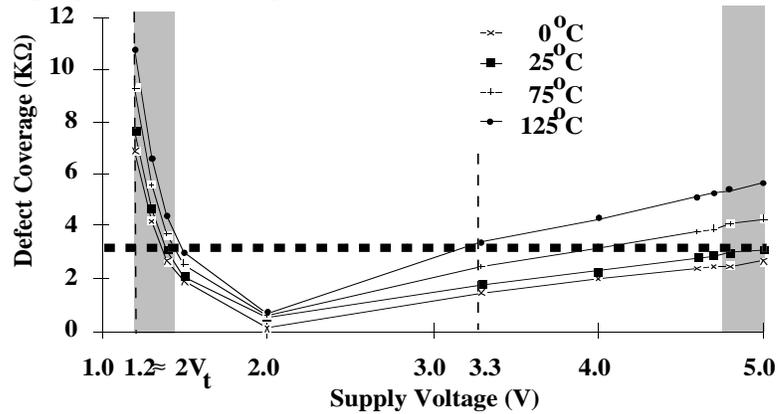
**Figure C-9 Desired Supply Voltage Range (in the Gray Region)**
