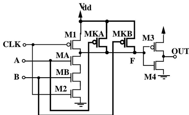
**Figure 4-7 2-input CMOS Domino AND Gate with Keeper Design A**
