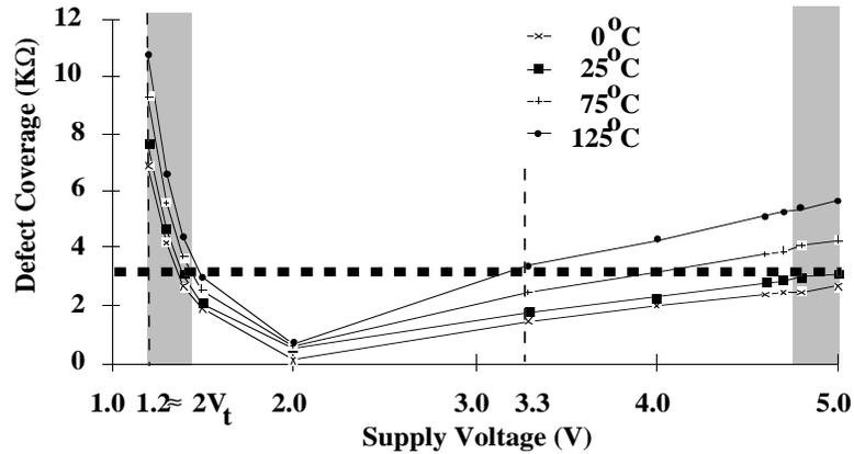
**Figure 4-6 Desired Supply Voltage Range (in the Gray Region)**
