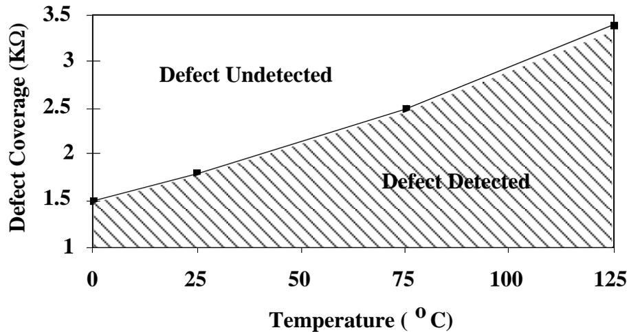
Figure C-7 Defect Coverage of the Short in Fig. C-6 at Different Temperatures for  $V_{dd} = 3.3V$
