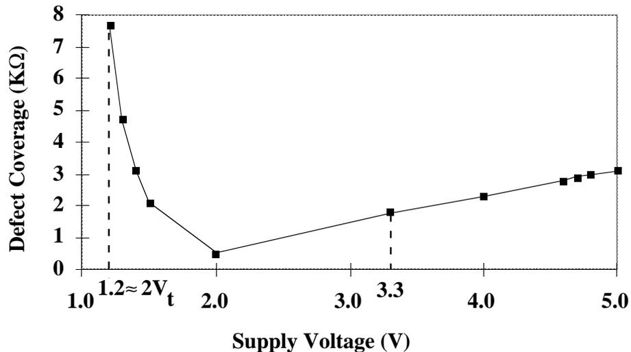
**Figure C-8 Defect Coverage of the Short in Fig. C-6 at Different Voltages for Temperature = 25°C**
