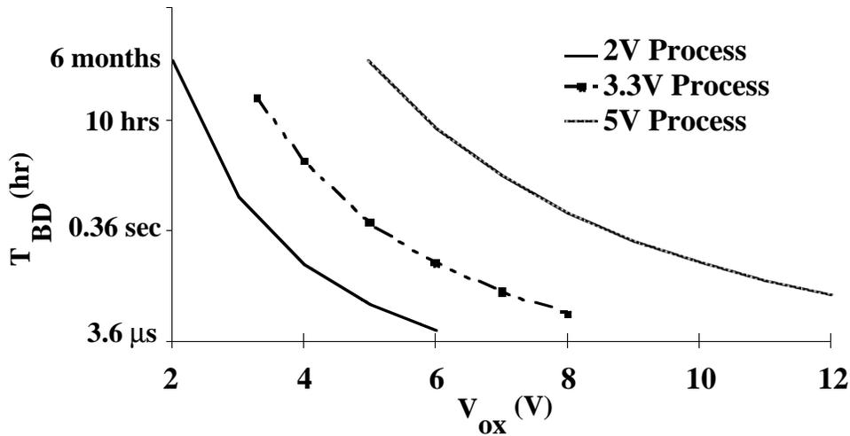
Figure 5-2 Lifetime of Defective Oxides (Thinner by 60%)
