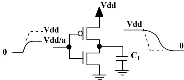
**Figure 3-1 Effect of a Degraded Signal**
