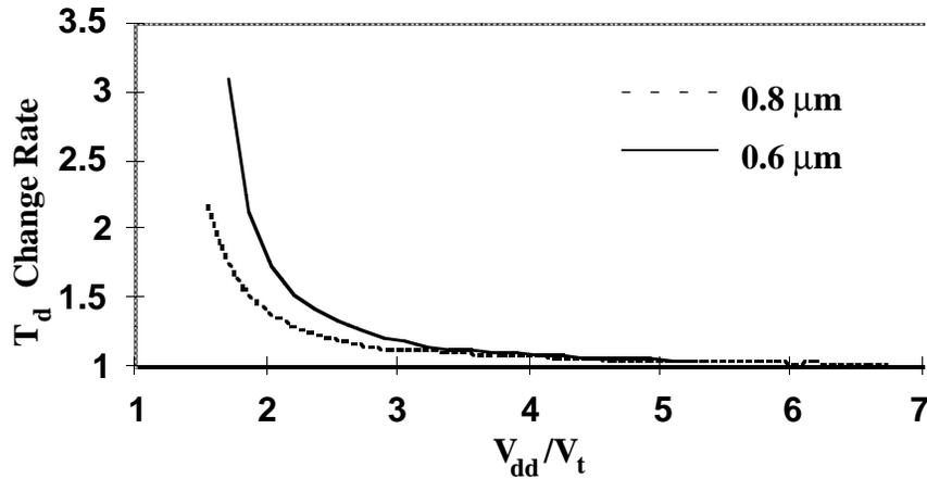
**Figure 3-2 Voltage Dependence of the Change Rate of the Propagation Delay of a CMOS Inverter**
