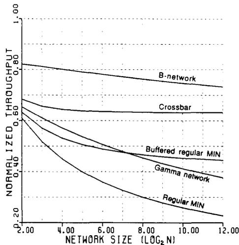
Fig. 5. Normalized throughput versus network size for various networks.
