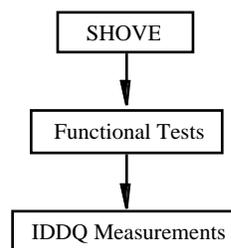
Figure 1 SHOVE testing procedure
