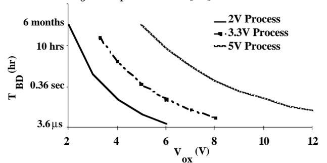
Figure 2 Lifetime of defective oxides for three different technologies
