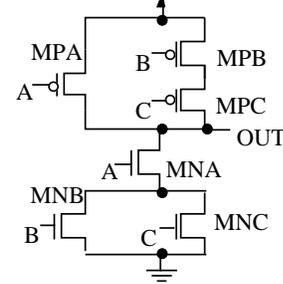
Figure 4 Fully complementary CMOS logic gate
