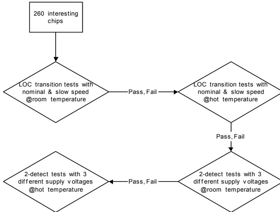
**Figure 10 NV2B Test flow**
