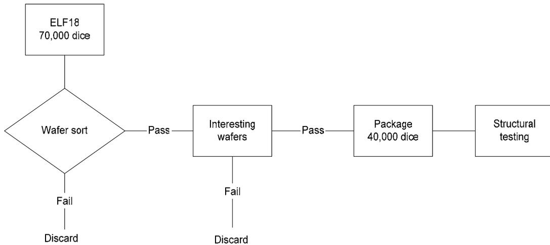
**Figure 15 ELF18 Test flow**
