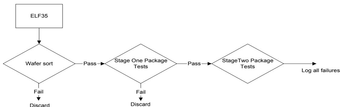
**Figure 14 ELF35 Test flow**
