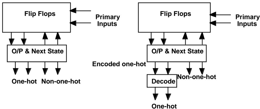
**Figure 1 :** General Structure of FSM      **Figure 2 :** Modified FSM to ensure 1-hots
