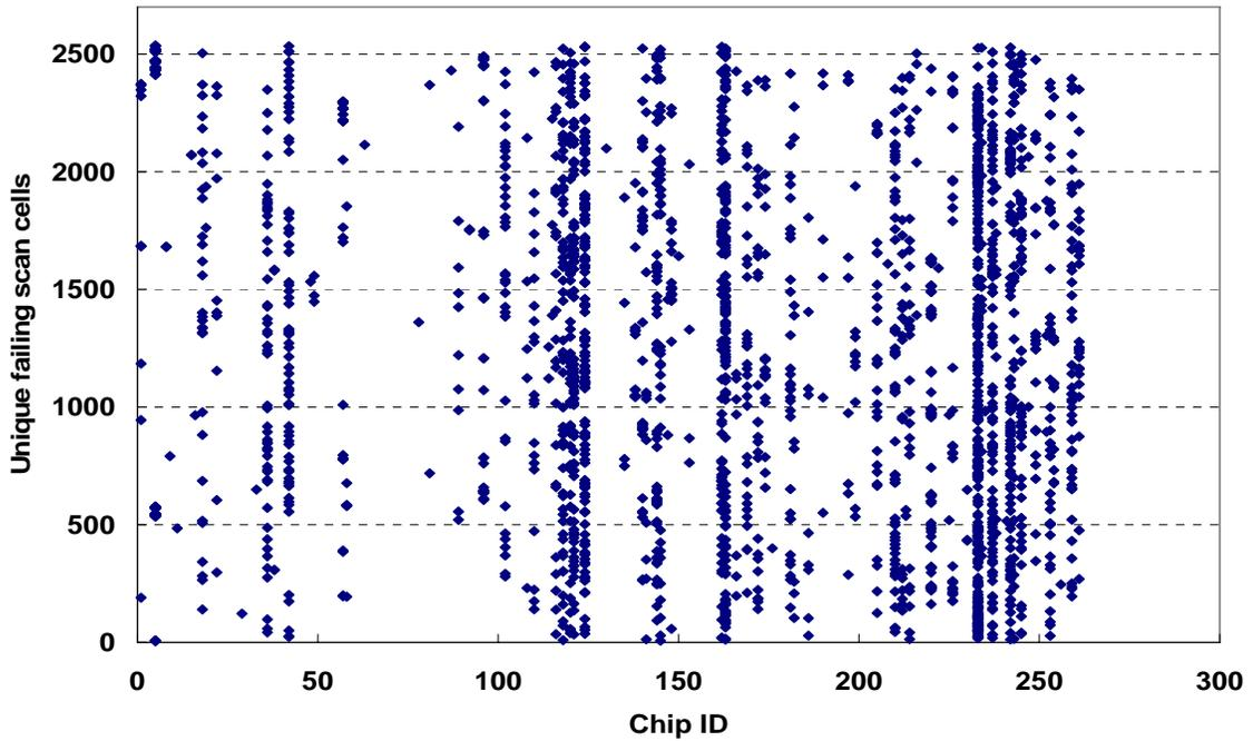
**Figure 9 Failing scan cell distribution of FP devices - ELF13**
