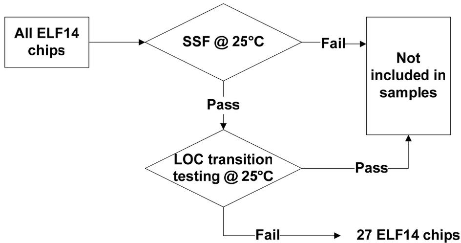
**Figure 2 ELF14 Production test flow**
