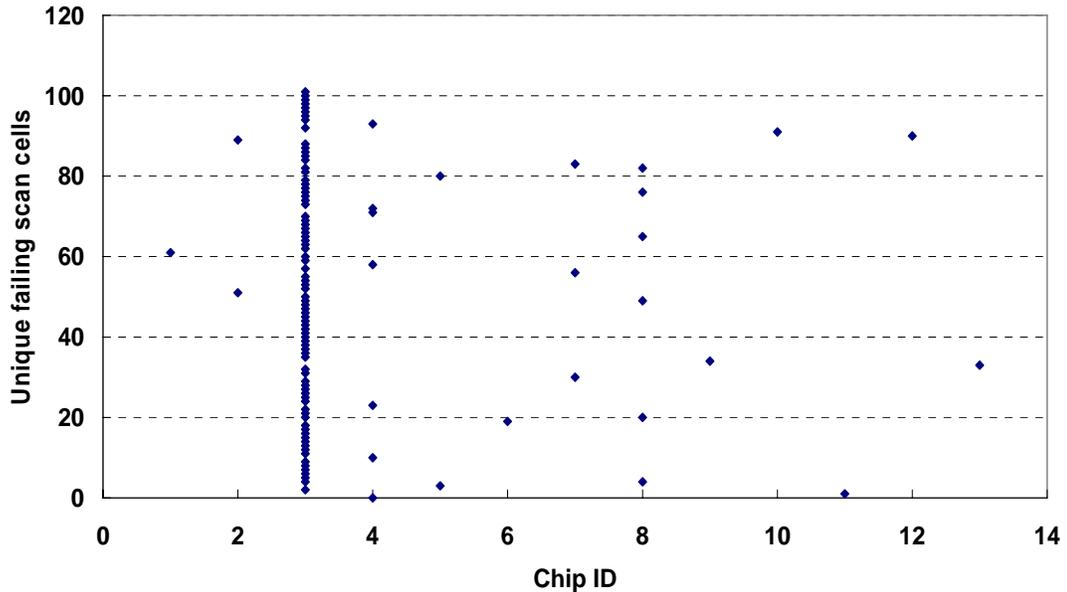
**Figure 8 Failing scan cell distribution of FP devices - ELF14**
