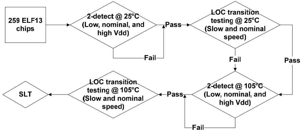
**Figure 5 ELF13 experiment test flow**
