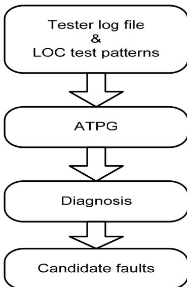
**Figure 12 Flow to obtain candidate faults**
