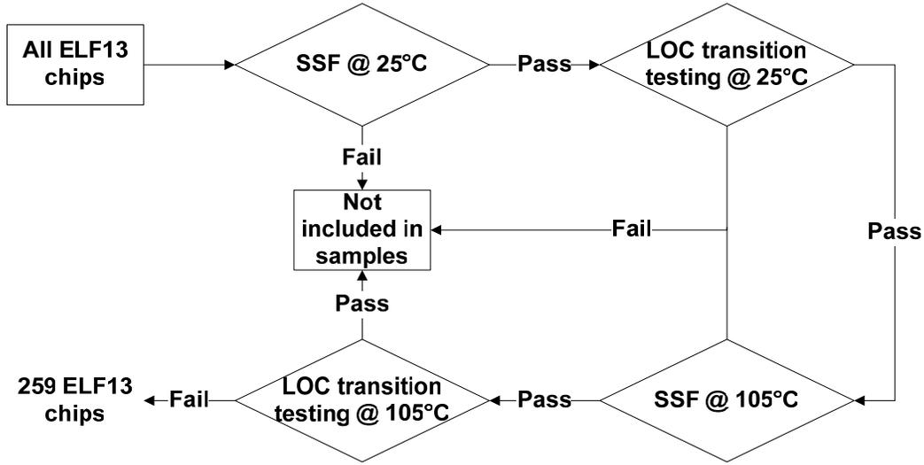
**Figure 4 ELF13 Production test flow**
