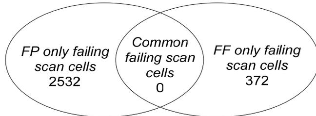
**Figure 7 Comparison of the number of failing scan cells for ELF13**
