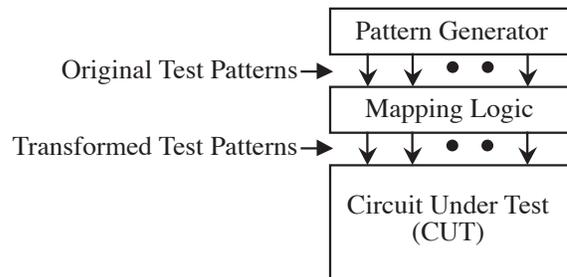
**Figure 1.** Block Diagram for Generation of Transformed Patterns
