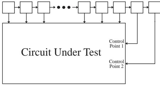
Figure 9. Control Points Driven by Extra Scan Elements
