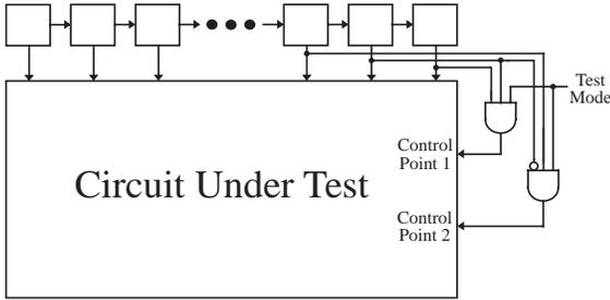
Figure 10. Control Points Driven by Pattern Decoding Logic
